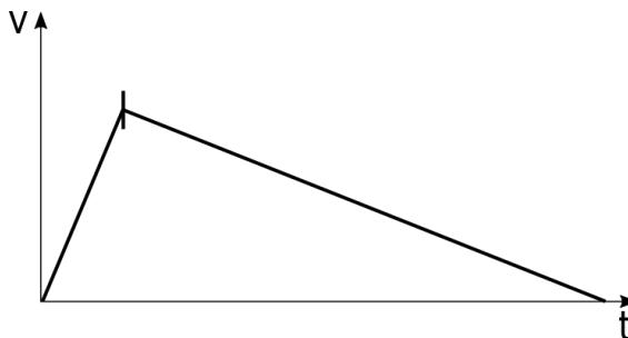
As there is no maximal velocity state, the *Measured Force* is not captured and therefore the *0V Raw Data Offset* does not change.
