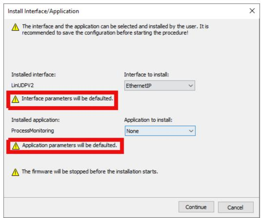
After clicking on the Continue button, LinMot-Talk logs out from the drive and install the selected firmware parts. When the installation is complete, LinMot-Talk logs in to the drive again. After the logging in the process is complete.
