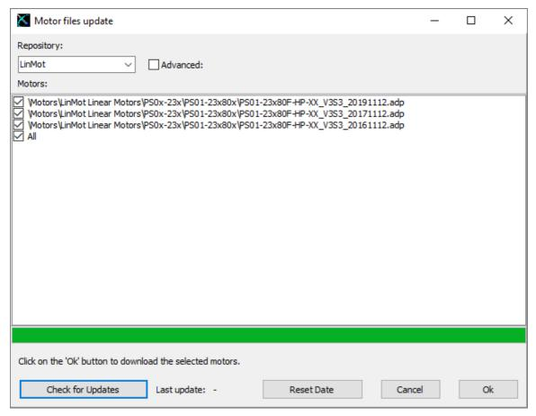
Each motor file has a date on which it was created. With this date it is possible to see how old your motor files are. With the option All, all motor files from the server will be downloaded. This option is normally only possible if the update date has been previously reset.
