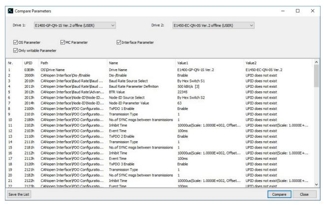
This useful function works with online and offline configurations. There are different setups available, such as firmware instances (OS, MC, INTF and APPL) or parameter types (read only or writable). The parameter list can be saved as a \*.pvl file (comma separated text file).
