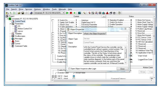
The Object Inspector window can be dragged away or closed. It can be reopened with F1. By login into a Drive without installing firmware before, it is possible that the firmware on the drive may not have the same version as LinMot-Talk. In this case it is possible to download the correct files to login. This is described in the chapter downloading Olderreleases.
