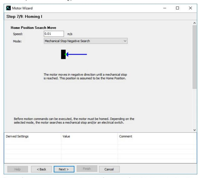
The most frequently used homing mode is "Mechanical Stop Negative Search". In this case the slider will move with the notch towards the stator's front end (where no cable is). Other modes support homing on home switches, limit switches, indexer inputs or some combinations of those.
