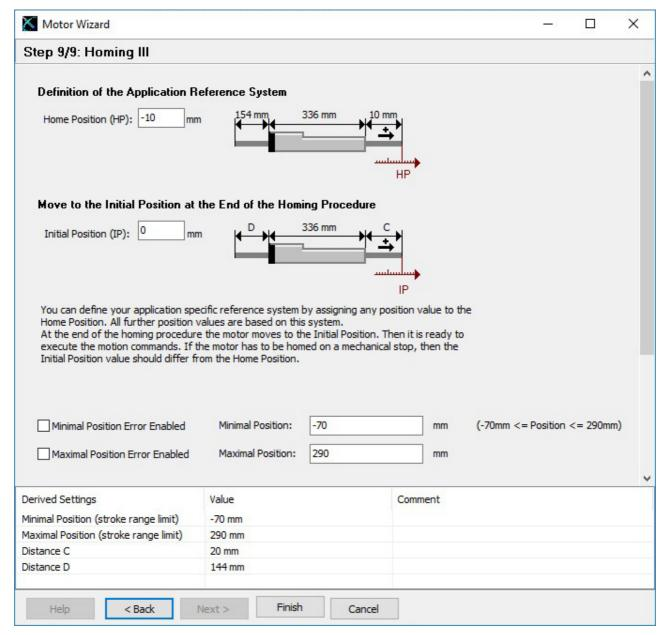
At the end, press finish. If the firmware on the drive is still running, an appropriate message will be shown. All parameters will now being written to the drive.
