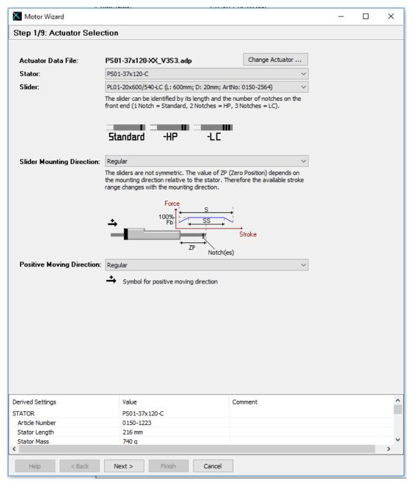
The derived settings show information about the complete motor type, article numbers and the most important technical data. The change of the positive moving direction is supported since release 6R7 and only for motors with PnP version V3S2 and higher. Motor with PnP version V3S1 do not work with changed positive moving direction. Be also aware in case of exchange!
