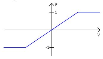
Demand Velocity: Means that the compensation will be made with the demand velocity and the table values will be multiplied by the factor F in the graph below. This is the recommended option and is set by default from by the wizard.
