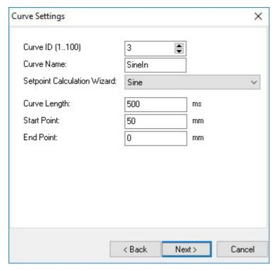
Set curve ID to 3, Curve Name to "SineIn", Curve Length to 500ms, Start Point to 50mm and End Point to 0mm. Click twice "Next" and then "Finish".
