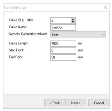
In this mask, we will set the curve ID to 2 (we will have the merged curve with ID 1 at the end) and as name we set e.g. "SineOut". The end point is placed at 50mm. With "Next" the wizard will show some curve data:
