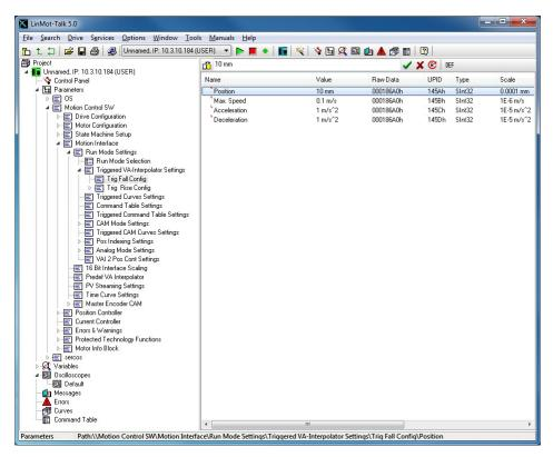
This is all we have to configure. The speed, acceleration and deceleration can also be defined at this place in the parameter tree. The motor can now be started the same way as described under 3.18.
