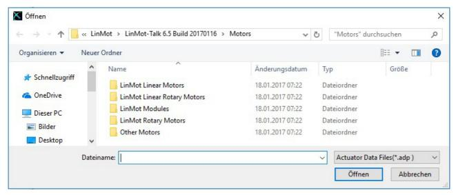
As we want to configure a LinMot Motor we choose "LinMot Linear Motors" and press Open. Then we choose the statorfamily like "PS0x-23x" and then the statorsubfamily like "PS01-23x160x". Select the actuator type you have connected to the drive, then press Open.
