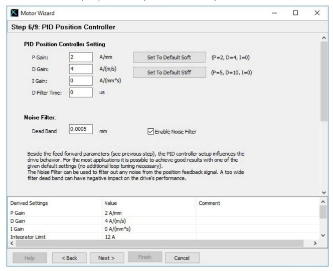
It is recommendable to start with the default soft settings, because the parameters can be changed any time later on (by restarting the motor wizard or by setting in the parameter tree directly).
