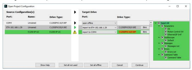
In this window, each configuration in the file has a line, in the combobox a drive could be selected. In this drive the configuration will be loaded. There are four possibilities of imports. They have the followed Symbols.
