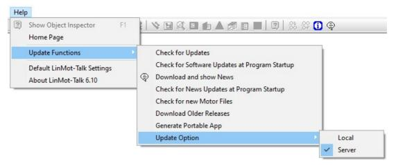
LinMot-Talk ask for the path of the packages. If both packages are needed, they must be on the same location. After that, LinMot-Talk try to update from the local path. In the error message when connecting the server, the button 'Change to local Package' directly changes the update option. It is possible that the packages have an older version then the data on the update server.
