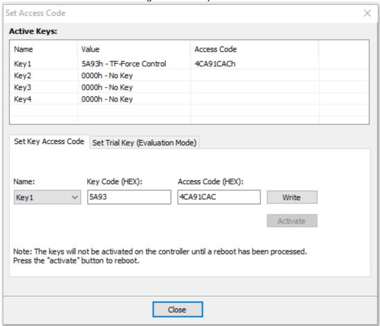
A maximum of four keys can be set on the drive. Under Active Keys all valid installed keys are listed (key value and access code).
