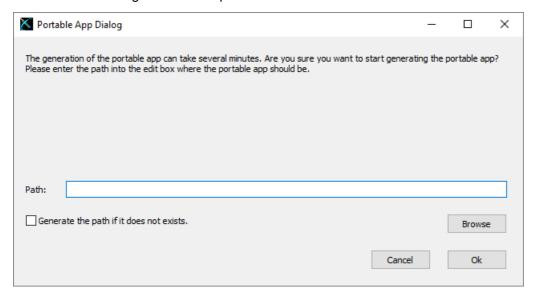
With "Browse" it is possible to choose the path of a folder. If the path is typed manual, with checking "Generate the path if it does not exists" it is possible to generate a new folder for the Portable App. By clicking on the Ok button and the path is correct, the LinMot-Talk copy's all necessary files into the folder. It is recommended to update the motor files and get all used olderreleases from the LinMot-Server before generate a portable app.
