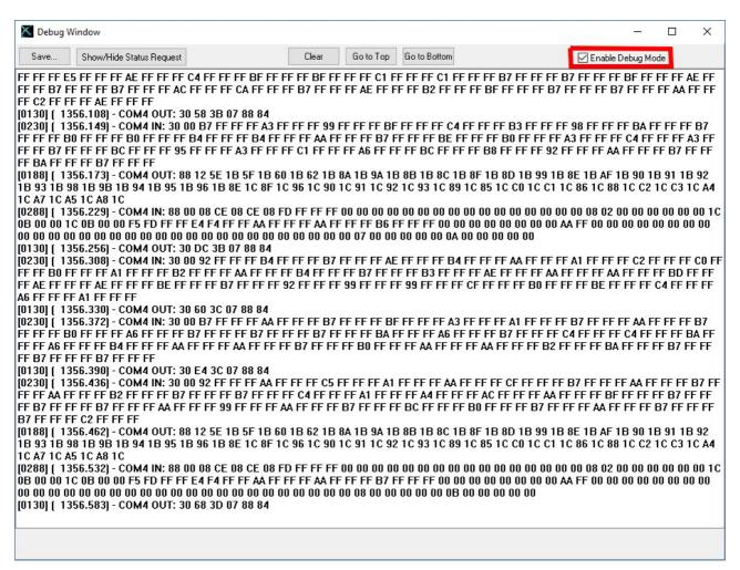
In the menu, Options – Save Debug Window Data, it is possible to enable the automatic save of the debug window.
