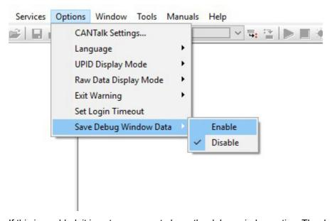
If this is enabled, it is not necessary to have the debug window active. The data will be saved in files with the path: "C:\Users\username\AppData\Local\LinMot\LinMot-Talk6.6-BuildXXXXXXXX\Communication". The LinMot-Talk saves this data in 10 files. It saves the data cyclic and when it begins with a new file it overwrites the oldest one. Every time when the LinMot-Talk will be restarted this option is disabled.
