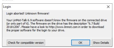
By clicking on the "Check for compatible version" button, LinMot-Talk search the correct files on the server and download them. When it finished in the text is written if the download was successful and after clicking the OK button, the LinMot-Talk ask if it should start the login process again.
