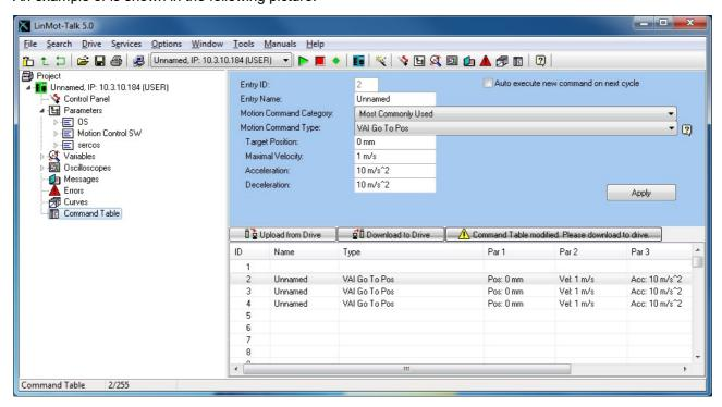
A big variety of commands can be set in this tables, such as motion commands, conditions, sequence directives, parameter access, ...
