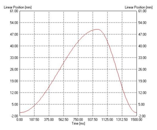
Now the curves must be downloaded to the drive. Therefore press the "Show Curves" button the "Download Curves into Drive" button be confirmed and the progress window will display the actions taken to download the curves.
