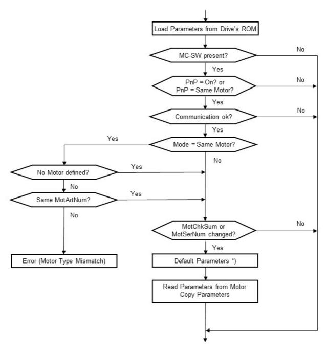
\*) All parameters, which are set by the previous PnP motor and do not exist in the new motor will be set to default values prior to load the new parameters.
