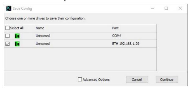
The selection Advanced Options opens the tree to select only parts of a drive. It can be selected for each drive different parts. The active drive is market green. To change the active drive only click on the new drive that should be active.
