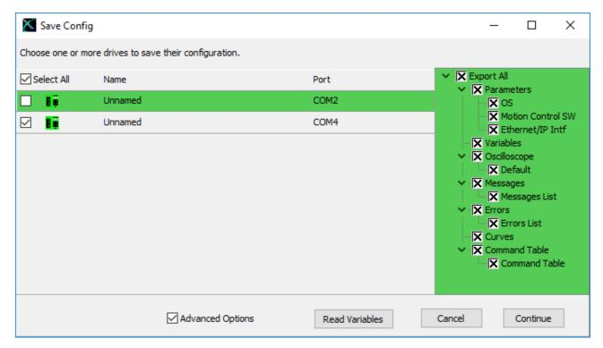
After that the file name dialog will open to choose the filename and the folder where the file should be saved. It is recommended to export all parts of a drive. For a configuration recovery, it is necessary to select the parameters, curves and command table.
