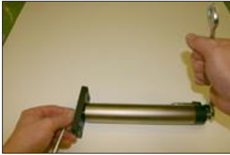
Incorrect assembly Torsional stress on slider
