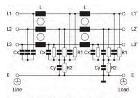
Note: HVIT versions without discharge resistor to ground.
