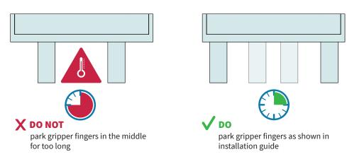
Detailed information and further operating instructions can be found in the gripper installation guide and data sheet at shop.linmot.com.
