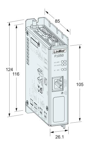
Dimensions in mm Mouting points for M4 screws
