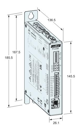
Dimensions in mm Mouting points for M5 screws
