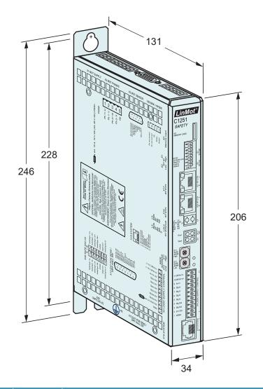
Dimensions in mm Mouting points for M5 screws
