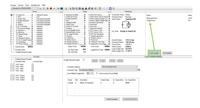
4. Now gently push or pull the linear axis. The variable "measured force" should rise or fall according to the variable "Motor Current".
