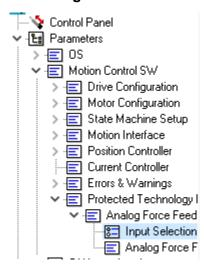
Logged into the drive, you will find all the parameters to be set in the LinMot-Talk software under the path "Parameters -> Motion Control SW -> Protected Technology Functions -> Analogue Force Feedback Control".
