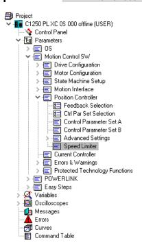
The maximum speed for force, torque and current control is defined under the "Speed Limiter" tab. If the parameterised speed "Speed Limit" is exceeded, the drive automatically switches to position control and regulates the current speed to the defined value. The "Speed Limiter Abort Force" parameter defines the measured value below which the drive switches back to force, torque or current control. If the "Speed Limit" parameter is set to 0 m/s, the function is deactivated.
