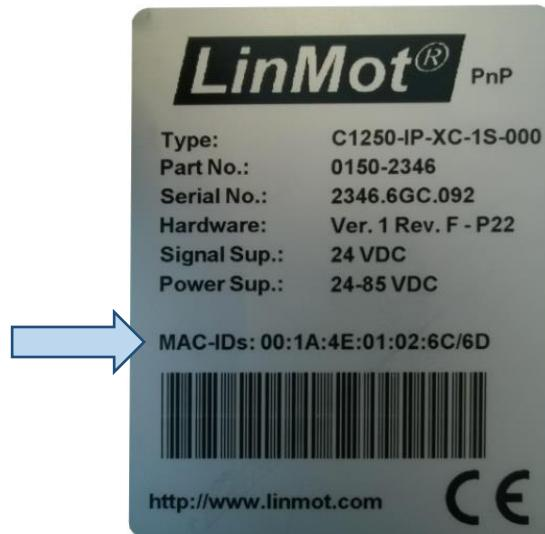
Select the correct MAC and assign the IP address to the drive.
