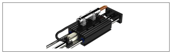
The flexible connector end of the M, C and R-cable type motors can be fixed with mounting clips. The clip is fixed to the guiding block with an M4x12 screw and an M4 square nut. In applications with a moving stator, the clips prevent damage caused by vibrations.
