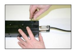
4. Tighten the clamping screws to the specified torque.
