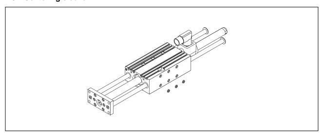
The centering sleeves simplify the mounting of the linear guide to another module. The mounting options of the linear guide are provided by several threaded holes at the bottom and side of the guide block.
