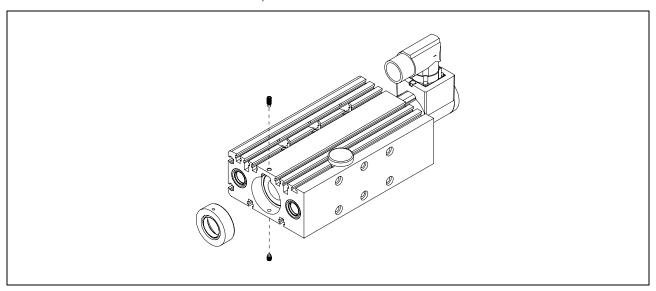
The wiper is fixed on the front side of the guide using 2 set screws (top / bottom). On the opposite side, a wiper is mounted at the end of the stator. This wiper is an accessory for linear motors.
