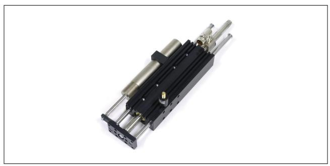
With a MagSpring installed parallel to the linear motor, the weight force can be compensated passively. In the de-energized state, this prevents the axis from lowering. Other possible applications are, for example, the generation of a contact force independent of position or the one-sided force assistance in drive tasks.
