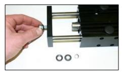
2. Place the spherical washer on the slider screw and insert it into the front plate.
