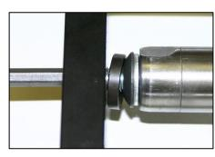
3. Place the conical seat, the spherical washer and the dished washer on the other side of the front plate onto the slider screw.
