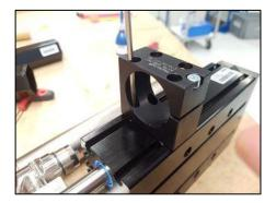
2. Place the flange on the guide block and tighten the screws slightly.
