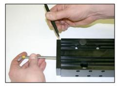
Completely retract the guide unit and then tighten the slider screw.
