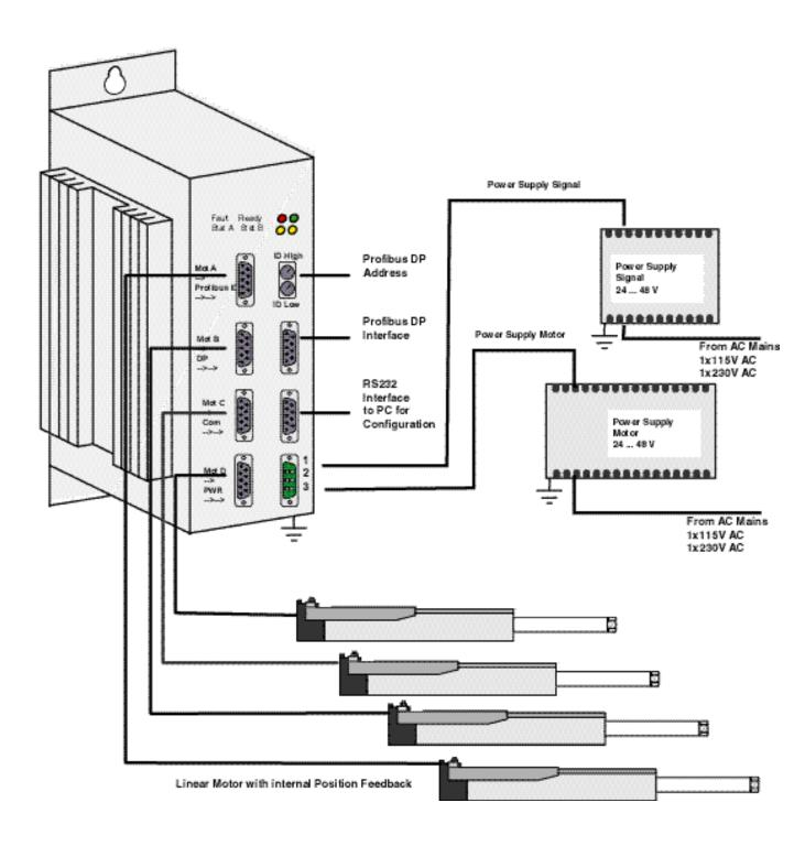
Complete E430 Controller based system (E130 and E230 controllers will only drive one respectively two motors). Power Supply for Signal and Motor may be the same device (see later).
