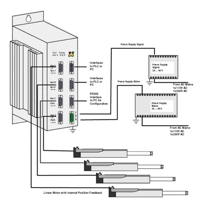
Complete E400 Controller based system (E100 and E200 controllers will only drive one respectively two motors). Power Supply for Signal and Motor may be the same device (see later).
