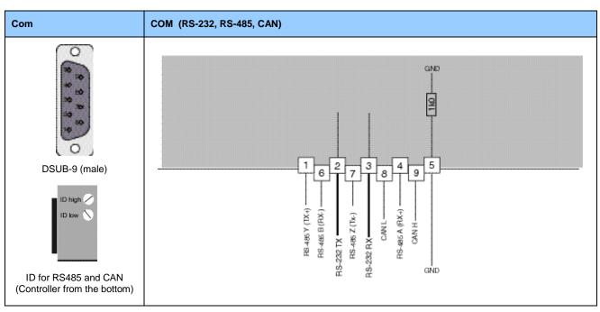
RS232: 9.6kBaud, use 1:1 connection cable to PC RS485 and CAN needs external termination (see manual)
