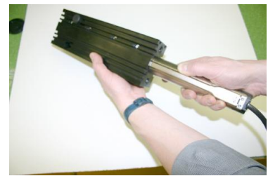
Insert Stator (clamping parts may have to be moved)
