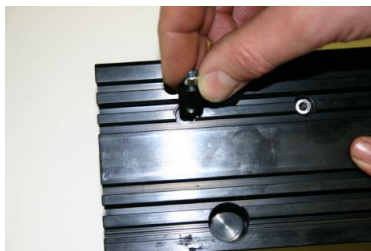
Place clamping elements into Guide Flange (do not tighten screws)
