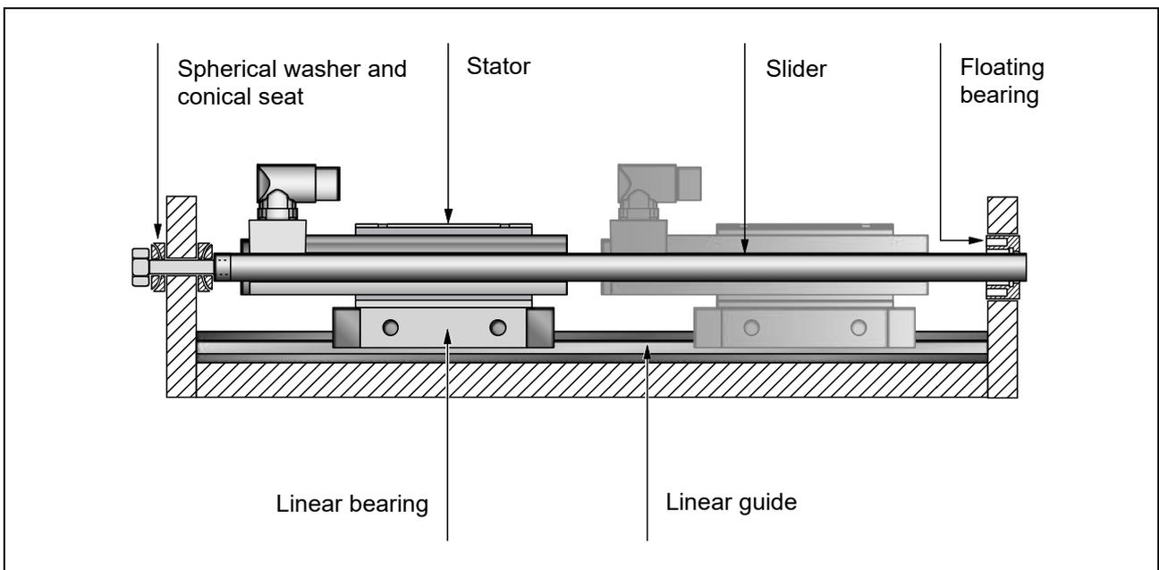
In "moving stator" applications, the slider is fixed and the stator is the moving part. The load is attached to the stator, which is mounted on a linear guide. In order to avoid an overconstrained bearing mount and compensate for alignment errors, the slider may be mounted on one end in a fixed bearing with a spherical axial bearing. On the opposite end, the slider is mounted in a floating bearing. Mounting kits are available for mounting the slider (see the section Slider mounting kits).
