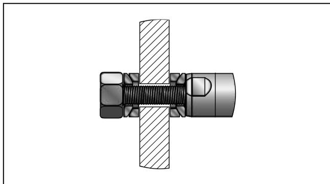
Slider mounting kit consists of a spring washer, a pair of spherical washers, and a pair of conical seats. It allows the slider to be fixed in the direction of motion. It also helps to compensate for radial and angle offset.
