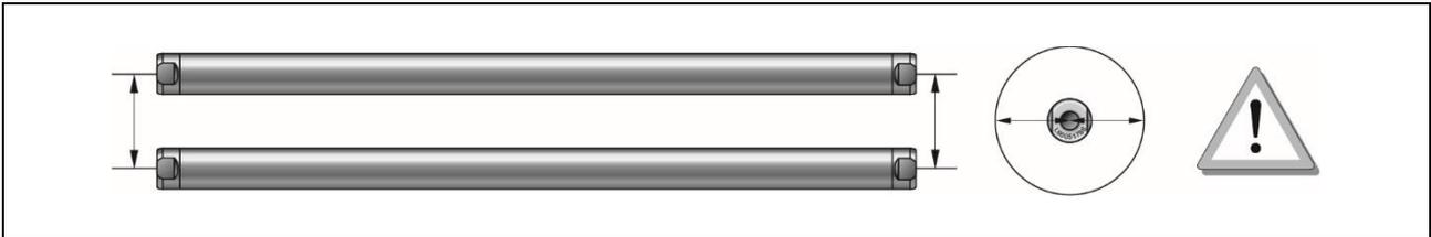
The sliders are made of neodymium magnets and have a strong magnetic attraction. It must be kept a minimum distance between the sliders. This minimized the risk of bruising and secondly, the sliders do not influence each other through their magnetic fields.
