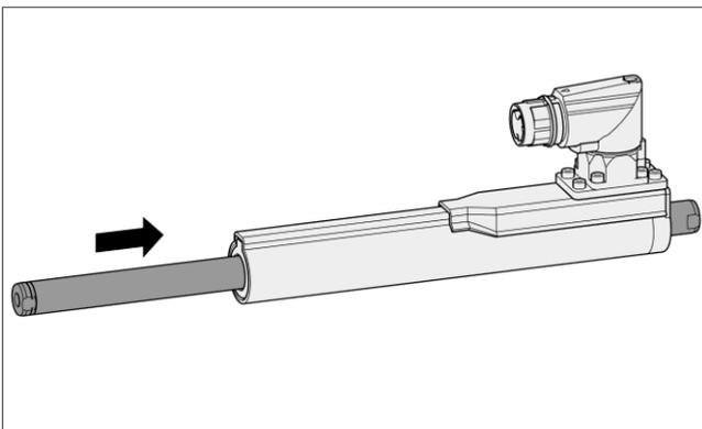
3. Insert the slider in the defined direction (see assembly step 4.).
