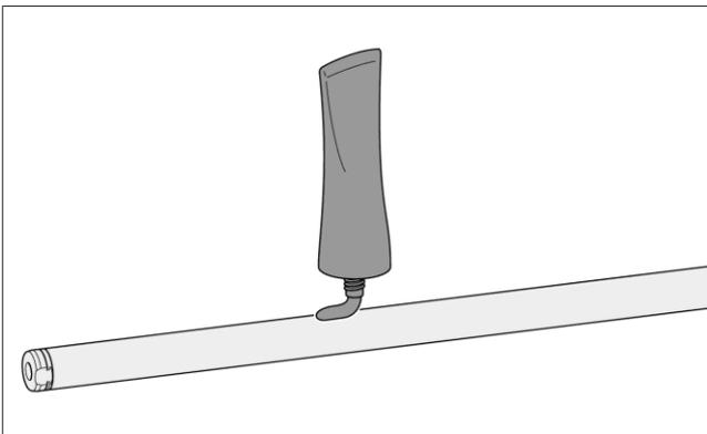
2. Lubricate the slider in accordance with the 'lubrication order' (see the section 6.3 Maintenance of linear motors)
