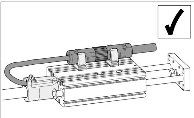
LinMot PS01-37x120-M stator in a moving stator application. The connectors are attached to the flange with the mounting clips. The cable attached to the motor is not moved and the minimum bending radius is maintained.
