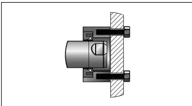
Floating bearing assembly that permits radial adjustment of slider position and permits a small amount of radial and axial movement.
