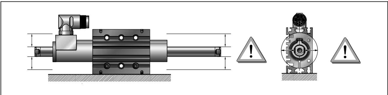
When installing linear motors in modules with metal parts near the slider, undesired forces can arise due to magnetic attraction or eddy currents. These generally manifest as erratic and jerky positioning, or reduced dynamics of the linear motor. In order to avoid this, minimum distances between the slider and any metal parts are to be observed whenever metal materials are used nearby.
