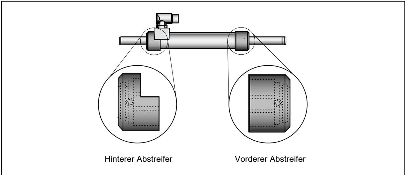
The stators are equipped as standard with wipers. This simplifies maintenance and the maintenance cycles can be extended. The wiper effects that the lubricant is dispensed metered and does not leak outside of the stator. The lubricant is less dirty.
