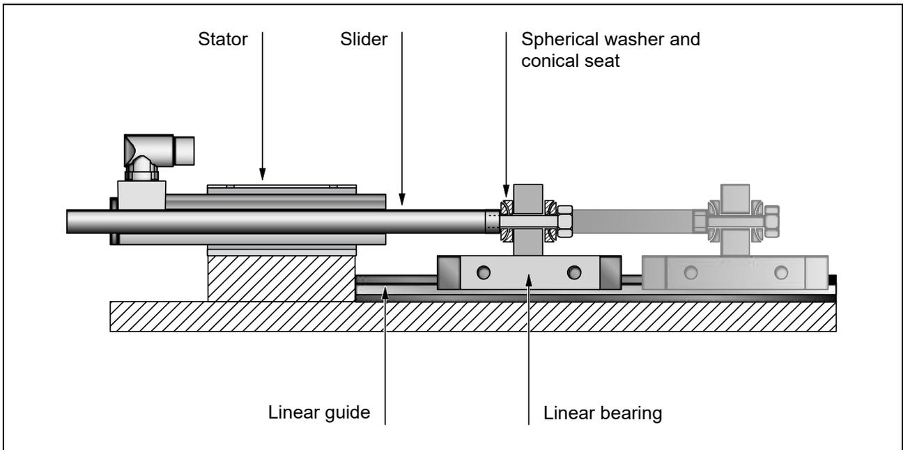
In a "moving slider" installation, the stator is fixed and the slider is the moving part. The load, borne by a linear guide, is attached directly to the end of the slider. In order to compensate for misalignment, spherical axial bearings consisting of spherical washers and conical seats (see the section Slider mounting kits) are used to connect to the load. The mounting kit of slider and an oversized hole for the screw make it possible to adjust a radial and angle offset.
