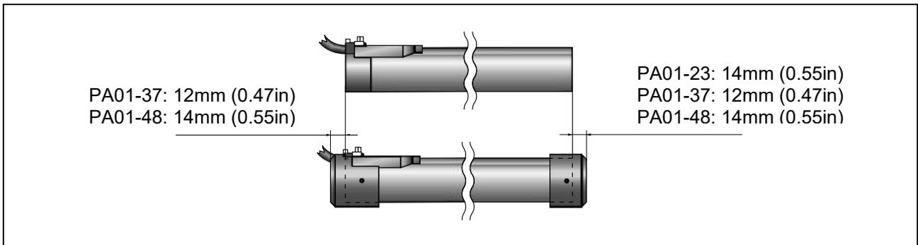
For each wiper, the lengthwise installation space for the stator, increases by 12 mm or 14 mm.
