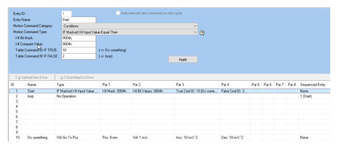
Line 1 is checking if the masked input corresponds with its bit value (same as bit mask) for proceeding in line 10, otherwise it loops via line 2 back into line 1.
