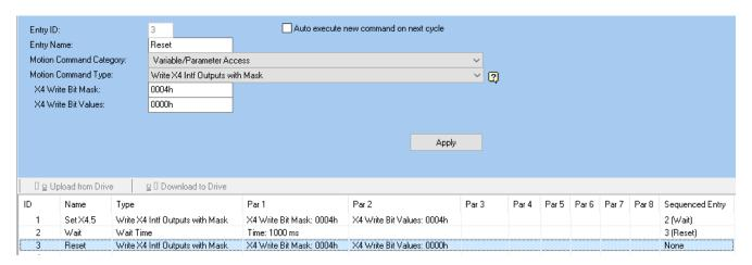
This example sets X4.5 to a high signal (on), wait 1s and reset X4.5 back to a low signal (off) and finish the command table.
