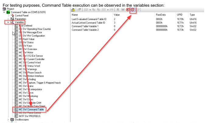
When the Command Table is running, you can observe both variables 1 & 2 and the actual linked line and the last linked line. This may be helpful to figure out which line sequence is working. This is especially helpful when "IF" conditions are used.
