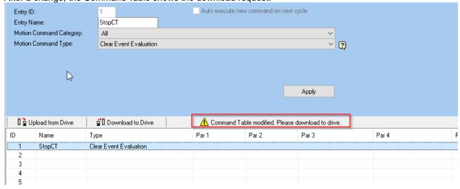
During download firmware must be stopped. When the download is complete, restart the drive.
